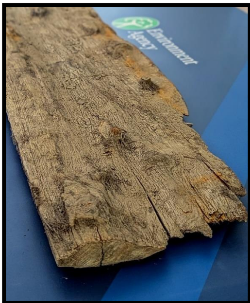
Cross section through one of the timber planks showing the deterioration which has eroded over many years.
